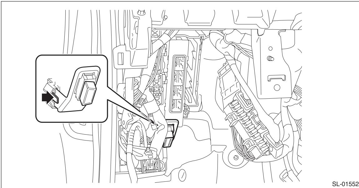
(3) Release the claws, and pull out the body integrated unit.
