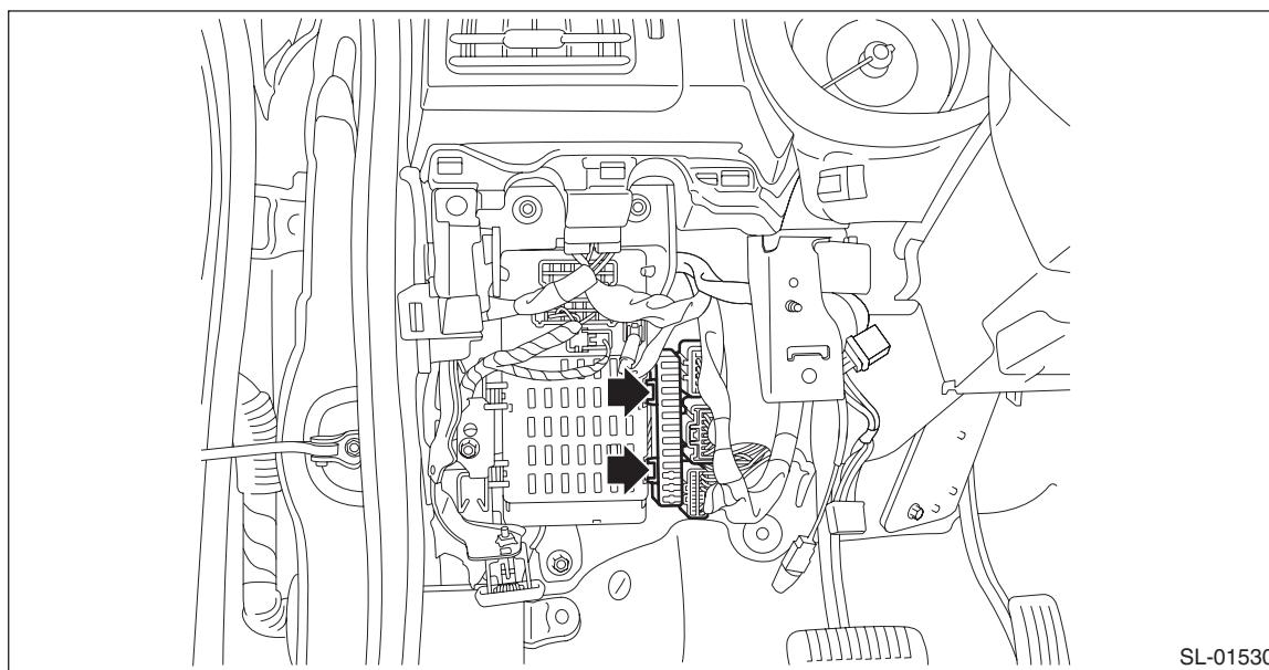
5) Remove the relay & fuse box.
